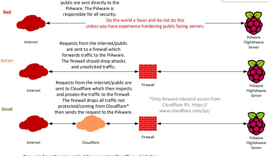
Requests from the internet/public are sent to Cloudflare which then inspects and proxies the traffic to the firewall. The firewall drops all traffic not protected/coming from Cloudflare\* then sends the request to an Apache Web Proxy that delivers the PiAware traffic to the requester. The PiAware never interacts with the public/requestor.
